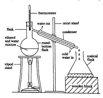
Ethanol has a boiling point of 78.5°C and water has a boiling point of 100°C. He found that the liquid collected in the conical flask boils in the range of 82-84°C.
