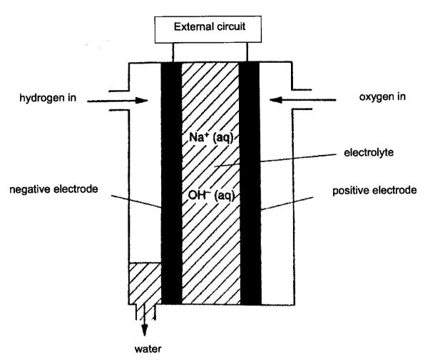
Complete the table below for the reactions that happen in the fuel cell. (a)
