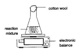
The rate of reaction was investigated by recording the mass of the reaction mixture at suitable time intervals.
