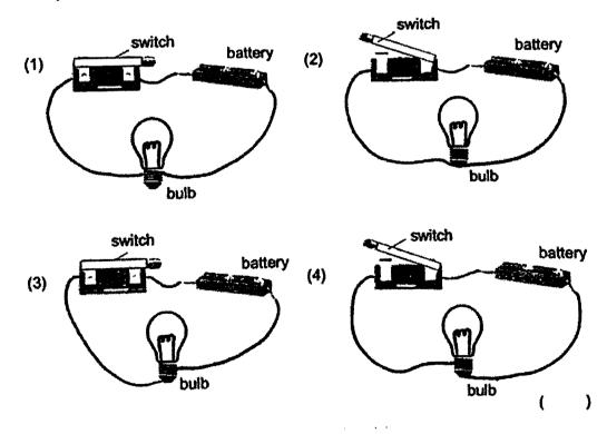
Peter set up an electrical circuit as shown in the diagram below. He closed the circuit with a coin and the light bulb lit. He repeated the experiment using different objects and wrote down his observations.
