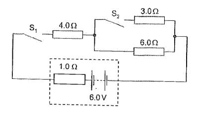
At time t = 0, switches  $S_1$  and  $S_2$  are closed.
