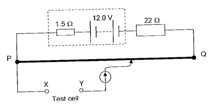
The wire PQ has a resistance of 3.0  $\Omega$  and the driver cell has an e.m.f. of 12.0 V. He was unable to obtain an observable balance length on PQ when he connected the circuit. The tutor he consulted told him that the test cell has an e.m.f. of a few millivolts. What could he do in order to obtain an observable balance length?
