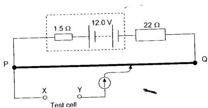
The wire PQ has a resistance of 3.0  $\Omega$  and the driver cell has an e.m.f. of 12.0 V. He was unable to obtain an observable balance length on PQ when he connected the circuit. The tutor he consulted told him that the test cell has an e.m.f. of a few millivolts. What could he do in order to obtain an observable balance length?
