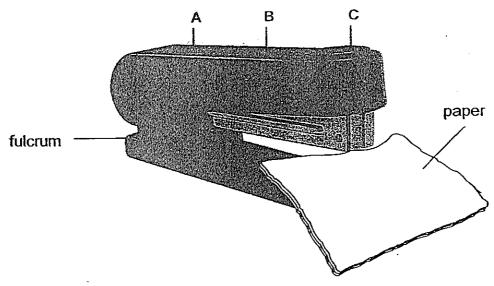
At which point of the stapler, A, B or C, will stapling of papers be made easiest?
