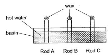
An equal amount of wax was placed at the top end of each of the three rods, A, B and C. The rods were then immersed in the basin of hot water at the same time.
