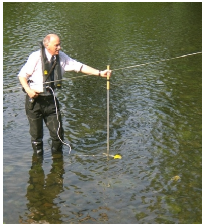
Flow meter used to measure velocity
