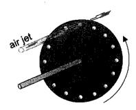
The time it takes for successive holes to move past the air jet is the period of the sound wave.
