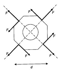
What is the net torque caused by all the forces?
