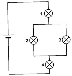
Bulb 3 is removed. Which of the following describes the changes in the brightness of bulbs 1, 2 and 4?
