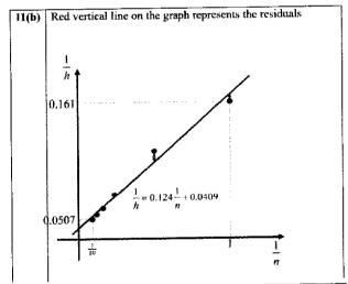
11 (c)  $h = \frac{an}{b+n} \quad \text{or} \quad \frac{1}{h} = \left(\frac{b}{a}\right)\left(\frac{1}{n}\right) + \frac{1}{a}$   $h = a - \frac{ab}{b+n} \quad \text{or} \quad \frac{1}{h} \to \frac{1}{a}$ As  $n \to \infty$ ,  $h \to a$  or  $\frac{1}{h} \to \frac{1}{a}$
